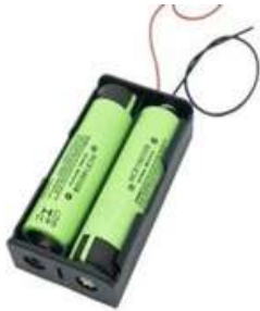
Figure 11. Battery Holder with Batteries
