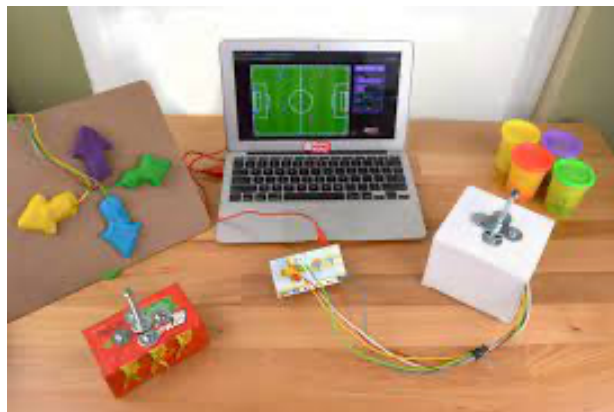
Makey Makey device connected to colored clay
